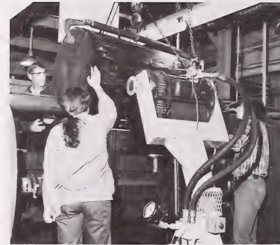
Forest Products Laboratory employees load a section of veneer log onto the lathe that will peel off the veneer. Ongoing experiments deal with increasing the amount of usable material from trees via improved logging and machining techniques.
